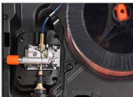
Kempact 181/251 models include the GT02C, two roll wire drive unit.
