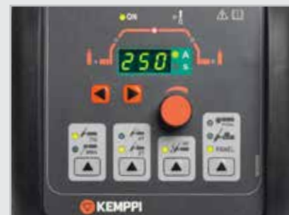
MasterTig LT 250 control panel: process selection for TIG and MMA, HF or Touch-Arc ignition, torch switch latching, and remote control selection. Current display, pre- and post-gas control, slope current timer.
