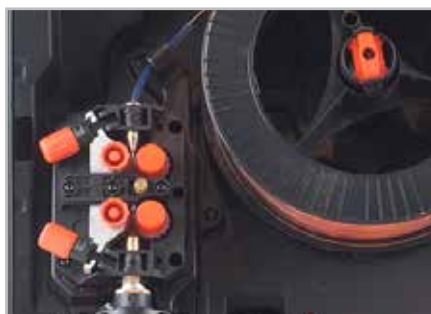
Kempact 253/323 models include the Dura-Torque four roll wire drive unit.
