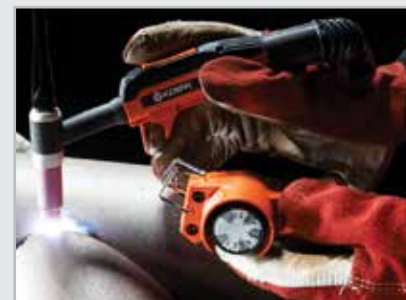
R 10 hand remote offers convenient current control at a distance, for both TIG and MMA process.
